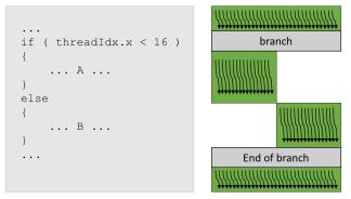
Visualization of divergent execution in Nvidia GPUs. Within a warp, if different groups of threads have to run separate code paths, then these code paths are taken sequentially.
